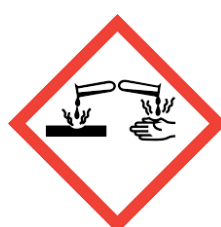
Figure 16: Danger pictogram for “Corrosive” (GHS05)
