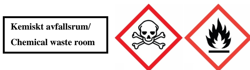
Figure 7: Recommended marking of waste sorting rooms where chemical waste is stored.
