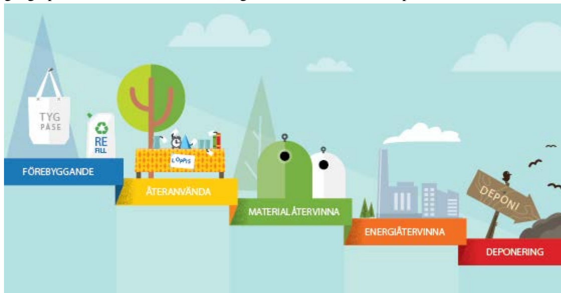
Figure 1: The EU's waste hierarchy/waste staircase shows that one must primarily prevent waste, thereafter strive for re-use, recycling of materials, energy recovery, and finally landfill (Source: http://www.sysav.se/skola/lararrum/Avfallstrappan/ ).
