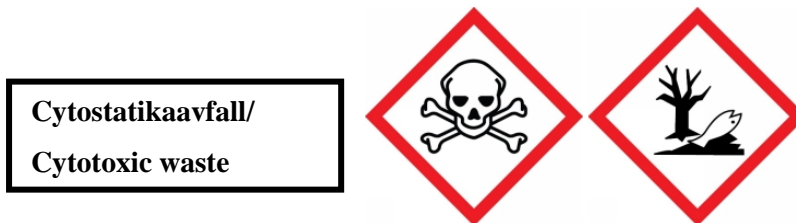
Figure 9: Recommended marking of waste sorting rooms where pharmaceutical waste covered by AFS 2005:5 on cytotoxic and other drugs with persistent toxic effect is stored.
